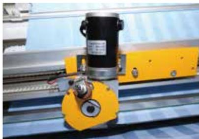
Intelligent cutting knife device: intelligent adjustable cutting device, blade loading and unloading is simple, self-carrying knife function to improve grinding knife effect.
