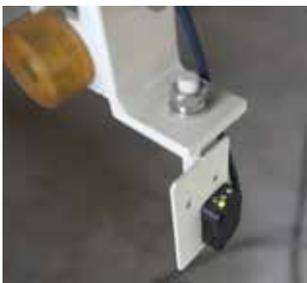
Spreading machine head is a moving part and may hurt operator or other people while they are near the machine, after the high sensitivity sensors are installed,the machine will stop immediately if anybody is close to the machine within 0.5M.
